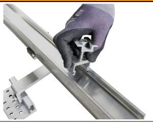
Place a module and slide it onto the CHRONOS middle clamp sets already clicked into place at the beginning of the rail. Make sure that there is a distance of 3.5 cm from the end of the profile.
