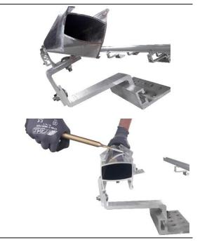
Screw at least two thin sheet metal screws (first and last CHRONOS roof adapter) per clicked-in profile into the hole pattern provided for this purpose on the back of the CHRONOS roof adapter in order to fix the CHRONOS Click profile. Use a hexagonal bit SW8 at a torque of 1 Nm.
