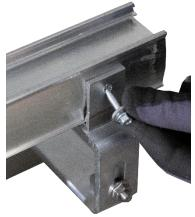
Slide the CHRONOS rail connector on to the end of the first profile at joints. Click the second profile into the rail con-4.5 nector (1). Then slide the rail connector over both profiles (2). Screw two thin sheet metal screws into the holes provided in the rail connector 4.6 (one screw in each end of the profile). Use a hexagon bit SW8 with a torque of 1 Nm. The first layer of CHRONOS Click Profile is 4.7 attached.
