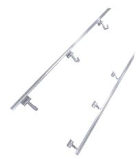
Insert or turn the M8x25 hammerhead screws into the bottom channel of the ZELOS profile. Insert the hammerhead screw through the hole patterns provided for the fastening points already attached to the roof. Place the ZELOS profile on the fastening points.
