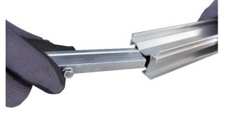
Slide the second profile onto the rail 4.5 connector. Now screw the profile that you have just attached to the rail connector to the roof fastening points according to 4.6 4.2 and 4.3. Repeat the above assembly steps for each row of profiles. The first layer of ZELOS profiles is 4.7 attached. 5 Optional: Mount the second layer of ZELOS profiles (for cross mounting). Measure the second profile layer and 5.1 mark it.
