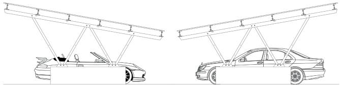
Example: Structure as trough roof arrangement ( $50x50 \text{ m} = 2.500 \text{ m}^2$ ; built-over area approx. 1.700 m<sup>2</sup>, access driving lanes with 3,85 m; 96 parking spaces, 6 x 16 double carports; 360 kWp, 936 modules 1.840 x 1.030 mm with 385 Wp each)
